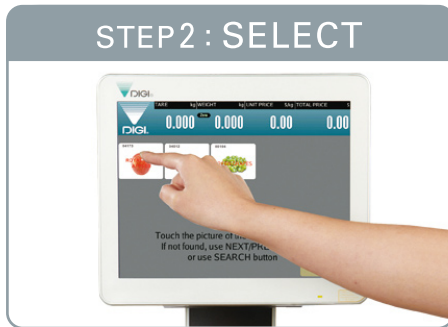
Select the correct icon. Camera recognises product and provides the closest match.
